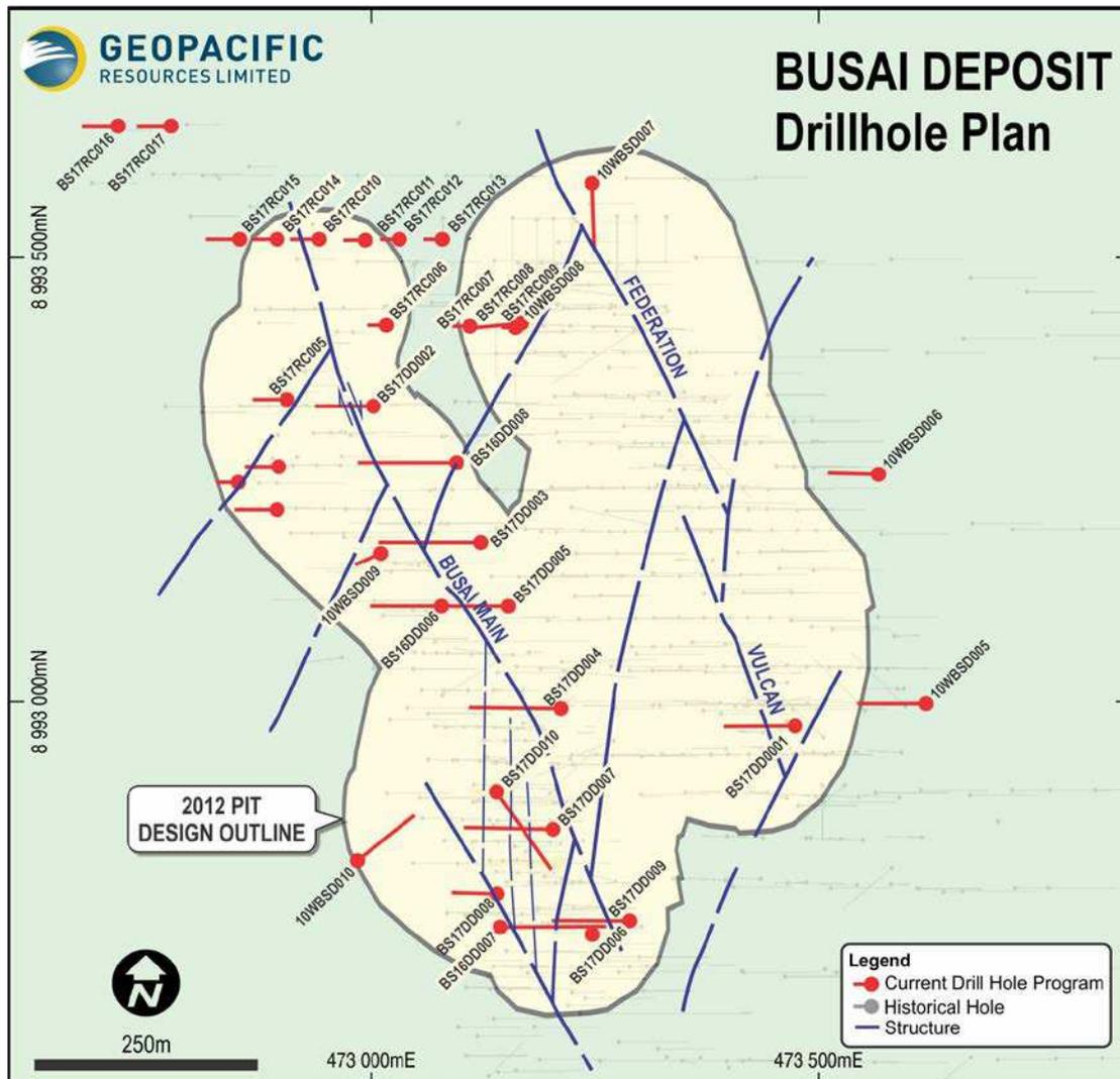
**Figure 5: Drillhole location plan at the Busai deposit**
